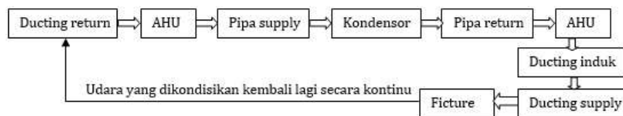
Gambar 8. Diagram Sistem Kerja Split Duct
