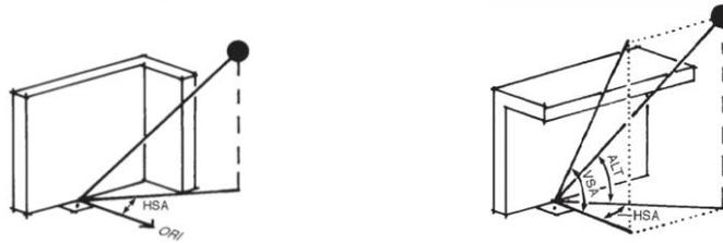
Gambar 1. *Horizontal Shadow Angle (HSA) & Vertical Shadow Angle (VSA)*
